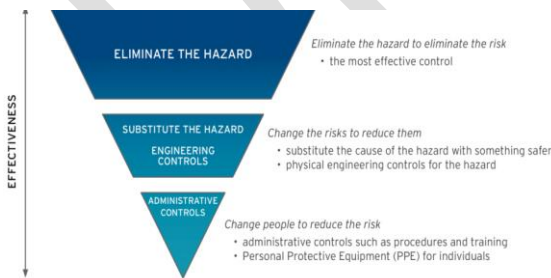
Figure (6). Hierarchy of controls for hazards and risks: demonstrating the approach required for risk management.
